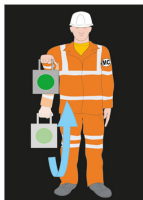
Slowly move away from the machine controller
